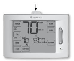
3) Insert Quick Reference Card into slot on top of thermostat.
