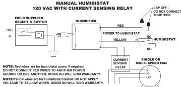
On furnaces where it is desirable to use a current sensing relay, the humidifier may be wired from a continuous 115 volt power source. Install the on/off switch in series with the hot or black wire. Install the Braeburn® 229050 Current Sensing Relay in series with the humidistat circuit. The Current Sensing Relay will detect furnace operation and supply power to the humidifier accordingly.
