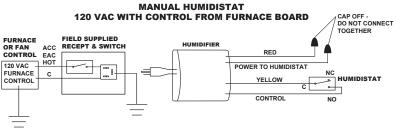
NOTE: Red wires are for humidistat power if required.
